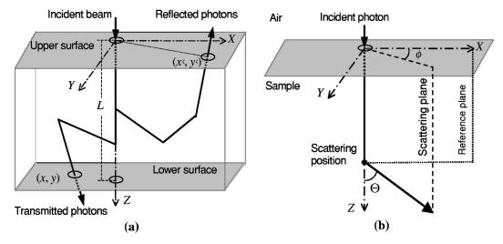
Fig. 2 (a) The geometry of multiple scattering events in a slab of turbid medium. (b) The geometry of the first scattering event during light propagation.
