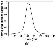
Fig. 1 (a) The schematic diagram of the experimental setup, where P is a polarizer, HW is a zero-order half-wave plate, QW is a zero-order quarter-wave plate, and A is a linear analyzer. (b) The response of the detection system to the laser pulse.
