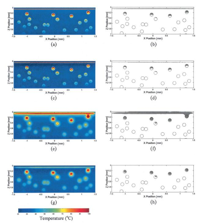
Fig. 10. False color temperature and skin damage maps for  $d = 120 \ \mu m$  and  $p_{mel} = 50\%$ . Four cases are shown: (a), (b)  $D = D_o$  for  $t_p = 0.5 \ ms$ ,  $t_{CSC} = 0 \ ms$ ; (c), (d)  $D = D_o$  for  $t_p = 0.5 \ ms$ ,  $t_{CSC} = 100 \ ms$ ; (e), (f)  $D = D_o$  for  $t_p = 20 \ ms$ ,  $t_{CSC} = 0 \ ms$ ; and (g), (h)  $D = D_o$  for  $t_p = 20 \ ms$ ,  $t_{CSC} = 100 \ ms$ .
