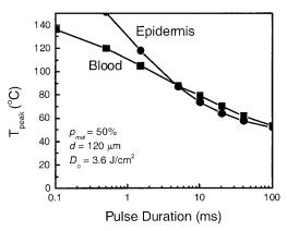
Fig. 6. Peak temperature  $T_{\text{peak}}$  generated within the blood vessel and epidermis versus pulse duration  $t_p$  for a constant radiant exposure.
