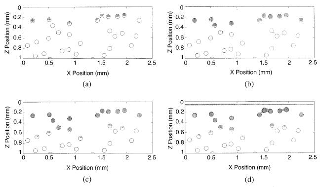
Fig. 5. Damage profile maps in skin for  $d = 80 \ \mu m$ ,  $t_p = 1.5 \ ms$ , and  $p_{mel} = 25\%$ : (a) no CSC and  $D_{th}$  (=3.1 J/cm<sup>2</sup>), (b) 50 ms CSC and  $D_{th}$  (=4.5 J/cm<sup>2</sup>), (c) 300 ms CSC and  $D_{th}$  (=6.6 J/cm<sup>2</sup>), and (d) no CSC with  $D = 6.6 \ J/cm^2$  [i.e. case (c) without CSC].
