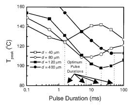
Fig. 8. Peak temperature  $T_{\text{peak}}$  within the epidermis immediately at the end of the laser pulse when the skin is irradiated at the therapeutic radiant exposure  $D_o$  versus laser pulse duration  $(t_p)$  for each vessel size in this study.
