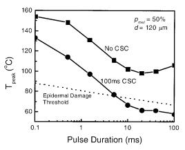
Fig. 9. Peak temperature  $T_{\text{peak}}$  within the epidermis immediately at the end of the laser pulse when the skin is irradiated at the therapeutic radiant exposure  $D_o$  versus laser pulse duration  $t_p$  for  $d = 120 \ \mu\text{m}$  without and with CSC ( $t_{\text{CSC}} = 100 \ \text{ms}$ ). Dashed curve, threshold temperature for epidermal damage ( $T_{\text{th}}$ ).
