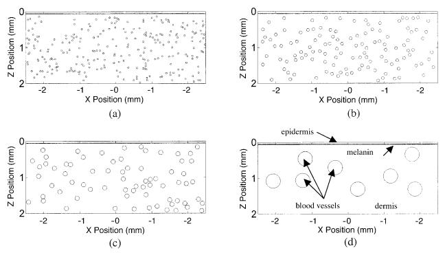
Fig. 2. Geometries used in this study. A 10- $\mu$ m-thick basal layer was located 60  $\mu$ m below the skin surface. Four vessel diameters [ $d = 40, 80, 120, 400 \mu$ m; (a), (b), (c), and (d) respectively] at their respective blood volume fractions ( $p_{bl}$ ) of 3.2%, 6%, 8%, and 10% were investigated.
