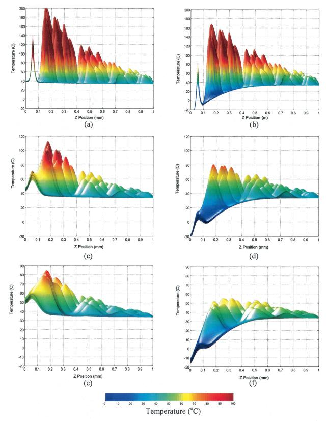
Fig. 4. Three-dimensional plots of the temperature, with the *x* direction coming out of the page, for a 1.5-ms laser pulse without [(a), (c), (e)] and with [(b), (d), (f)]  $t_{\rm CSC} = 300$  ms. Temperature profiles are shown immediately [(a) and (b)], 5 ms [(c) and (d)], and 10 ms [(e) and (f)] following the laser pulse.
