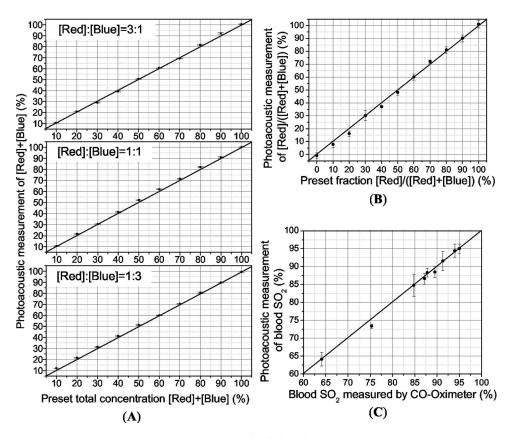
**Fig. 3** Photoacoustic measurement of (A) the total dye concentration, [red]+[blue], in each mixed dye solution containing Fiesta Red and Lake Placid Blue, where the ratios between [red] and [blue] are 3:1, 1:1, and 1:3, respectively, in the three charts; (B) the fraction of the red dye concentration in the total dye concentration, [red]/([red]+[blue]), in each mixed dye solution; and (C) the oxygen saturation of hemoglobin (SO<sub>2</sub>) in rat blood samples *in vitro*.
