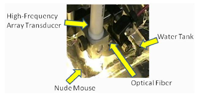
**Figure 2.** (1.8MB) Video of the realtime photoacoustic imaging system and realtime display while imaging the beating heart of an athymic nude mouse.
