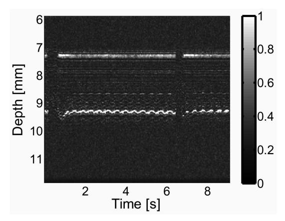
Figure 4. M-mode image along the X=0 mm line in Fig. 3. The oscillating structures around the 9-mm depth below the transducer surface show the cardiac motion as a function of time. The animal's heart estimated here as  $\sim$ 3 beats per second corresponded well to the 180 beats per minute as measured by the pulse oximeter.
