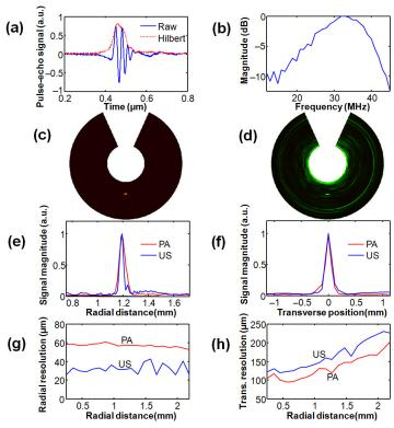
Fig. 3. (a) Typical US pulse-echo A-line signal of a tungsten wire: raw data and Hilberttransformed or enveloped signal. (b) Acoustic frequency distribution of the waveform shown in (a). (c, d) PA and US B-scan images of a 20-µm thick tungsten wire. (e) PA and US radial point-spread-functions (PSFs) of the tungsten wire. (f) PA and US transverse PSFs of the tungsten wire. (g) Radial resolution vs. target distance. (h) Transverse resolution vs. target
