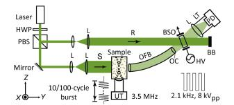
**Fig. 1** Schematic of the experimental setup. The component labels are defined as follows: HWP, half-wave plate; PBS, polarizing beam splitter; L, lens; S, signal beam; R, reference beam; UT, ultrasound transducer; OFB, optical fiber bundle; OC, optical condenser; BSO, Bi<sub>12</sub>SiO<sub>20</sub> photorefractive crystal; HV, high voltage electric field; BB, beam block; LT, lens tube; PD, photodiode detector; *XYZ*, system coordinates.
