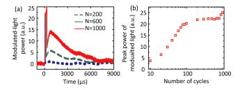
**Fig. 3** (a) Modulated-light powers corresponding to ultrasound bursts with 200, 600, and 1000 cycles, respectively. (b) Peak power of modulated light as a function of ultrasound burst length varied from 10 to 1000 cycles.
