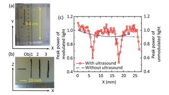
**Fig. 6** (a) Photograph of the 9.4 cm-thick phantom in the *XY* plane. (b) Photograph of the cross-section of the phantom at the central *Y* plane (Y = 4.7 cm). (c) Peak power of the modulated-light along the *X* direction. Measured peak power of the unmodulated-light distribution without ultrasound modulation is also included (blue dashed curve) for comparison.
