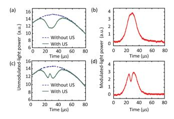
**Fig. 2** Examples of detected unmodulated-light power transmitted through a 6 cm-thick phantom with the embedded absorption object (a) outside and (c) inside the ultrasound beam, in the form of 10-cycle bursts. The difference between signals obtained without and with ultrasound modulation gives the ultrasonically modulated-light power shown in (b) and (d), respectively.
