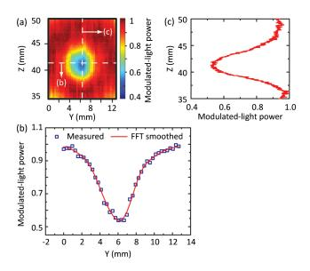
**Fig. 5** (a) UOT image at the central *X* plane for Obj1 [X = 6.4 mm] plane in Fig. 4(b)], where the positive *Y* axis is the signal beam incident direction. Modulated-light power distributions along the horizontal and vertical dashed lines in (a) are given in (b) and (c), respectively.
