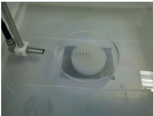
Fig. 2 A photograph of the pencil leads held in agar and surrounded by an acrylic cylindrical shell.
