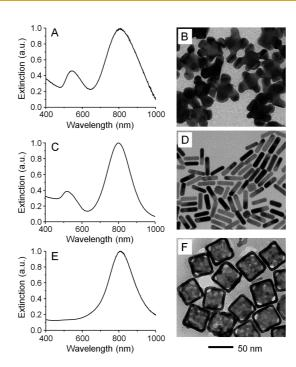
Figure 1. UV—vis spectra taken from aqueous suspensions of (A) Au nanohexapods (0.18 nM in particle concentration or 34.4  $\mu$ g/mL of Au atoms), (C) Au nanorods (1.4 nM in particle concentration or 36.4  $\mu$ g/mL of Au atoms), and (E) Au nanocages (0.024 nM in particle concentration or 9.6  $\mu$ g/mL of Au atoms and 3.3  $\mu$ g/mL of Ag atoms). (B, D, F) TEM images of the corresponding Au nanostructures. The 50 nm scale bar applies to all images.
