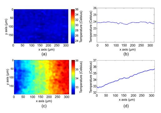
FIG. 3. 2D temperature mapping of a thin layer of Rhodamine 6 G dye. The phantom sample was heated at the right end. The FAPT-recovered temperature mapping (a) before and (c) after heating. Vertically averaged temperature profile along the horizontal direction (b) before and (d) after heating.
