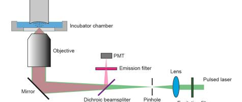
FIG. 1. FAPT system set up. The fluorescence and PA signals were measured simultaneously at each scanning point. PMT: Photomultiplier tube.
