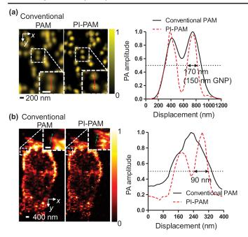
FIG. 3 (color online). PI-PAM imaging of gold nanoparticles and melanoma cells with enhanced lateral resolution. (a)–(b) 150-nm diameter gold nanoparticles (a), and a B16 melanoma cell (b) imaged by conventional PAM (left column) and PI-PAM (middle column). The normalized signal amplitude profiles along the dashed lines are shown in the right column. Insets show magnified views of the marked areas. The scale bars for the insets are 200 nm.
