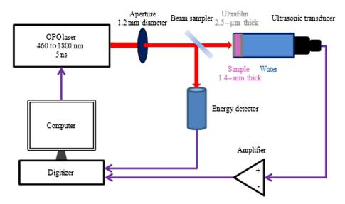
Fig. 1 Schematic of the photoacoustic spectroscopy system.
