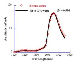
**Fig. 5** Typical photoacoustic spectrum of bovine serum. The normalized amplitude (mean  $\pm$  SE) is plotted versus wavelength. The solid curve is a fit to the absorption spectrum of 92% water, yielding the Grüneisen parameter to be 0.13.
