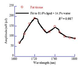
**Fig. 4** Typical photoacoustic spectrum of porcine subcutaneous fat tissue. The normalized amplitude (mean  $\pm$  SE) is plotted versus wavelength. The solid curve is a fit to the absorption spectrum of 81.6% lipid and 14.1% water, yielding a Grüneisen parameter of 0.79.
