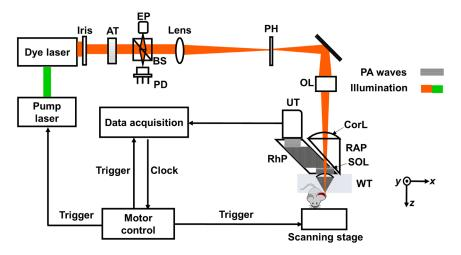
**Fig. 1** Schematic of photoacoustic microscopy (PAM) system. AT, attenuator; BS, beam splitter; CorL, correction lens; EP, eyepiece; OL, objective lens; PD, photodiode; PH, pinhole; RAP, right-angle prism; RhP, rhomboid prism; SOL, silicone oil layer; UT, ultrasonic transducer; WT, water tank.
