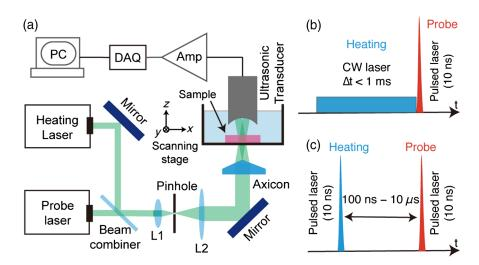
**Fig. 1** Schematic of Bessel-beam photoacoustic microscopy (PAM). (a) Experimental system setup. L1, L2: lens. (b) Continuous wave (CW)-heating scheme. A CW laser is used as the heating laser. The heating duration ( $\Delta t$ ) of the CW laser must be less than the thermal relaxation time. (c) Pulsedheating scheme. Both the heating and probe laser beams are pulsed, and the interpulse delay ranges from 100 ns to 10  $\mu$ s.
