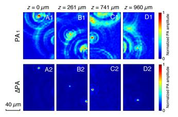
**Fig. 6** 2-D image slices from a volumetric image of a 1-mm-thick RBC sample in agar medium. Upper row: regular Bessel-beam PA images (PA<sub>1</sub>). Lower row: nonlinear Bessel-beam PA images ( $\Delta$ PA). Images at relative axial depths (a1 and a2)  $z=0~\mu$ m, (b1 and b2)  $z=261~\mu$ m, (c1 and c2)  $z=741~\mu$ m, and (d1 and d2)  $z=960~\mu$ m. The maximum signal amplitude was normalized to be 1 in each image.
