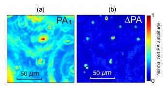
**Fig. 5** 2-D maximum amplitude projected (MAP) volumetric image of a 400- $\mu$ m-thick RBC sample in agar medium. (a) Linear Bessel-beam PA image (PA<sub>1</sub>) acquired without heating laser. (b) Nonlinear Besselbeam PA image based on the differential PA image ( $\Delta$ PA).
