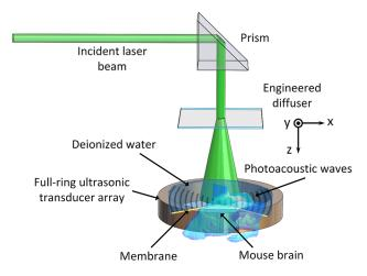
Fig. 1 Schematic of full-ring PACT system.
