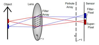
**Fig. 7.** Optical setup of an imaging spectrometer using a light field architecture. *u*, *v*, coordinates at the lens aperture; *s*, *t*, coordinates at the pinhole array. Source: Figure reprinted with permission from [60].
