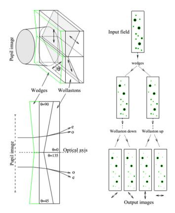
**Fig. 25.** Imaging polarimetry using a wedged double Wollaston prism. *Source:* Figure reprinted with permission from [218].
