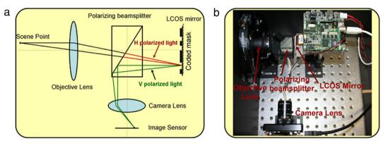
Fig. 23. Programmable pixel compressive camera (P2C2). a. Optical setup. b. Photograph of system. LCOS, liquid crystal on silicon. *Source:* Figure reprinted with permission from [13].
