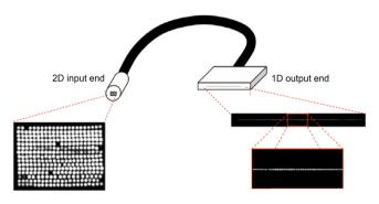
**Fig. 5.** Reformatting a 2D image to 1D signals by a maneuverable coherence fiber bundle. *Source:* Figure adapted with permission from [55].
