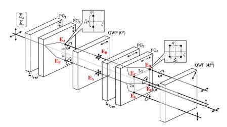
**Fig. 28.** Optical setup of a white-light channeled imaging polarimeter. PG<sub>1</sub>, PG<sub>2</sub>, PG<sub>3</sub>, PG<sub>4</sub>, polarization gratings; QWP, quarter-wave plate. *Source:* Figure reprinted with permission from [232].
