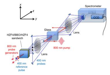
**Fig. 19.** Schematic setup for frequency-domain streak tomography of evolving pump-laser-induced refractive index changes. *Source:* Reprint with permission from [199].
