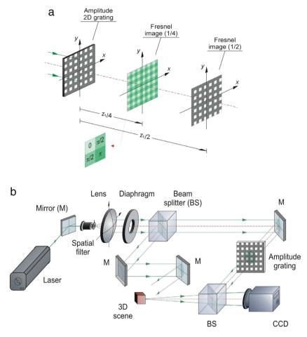
**Fig. 17.** Parallel phase-shifting digital holography utilizing the fractional Talbot effect. a. Formation of Fresnel images. b. Optical setup. *Source:* Figure reprinted with permission from [175].
