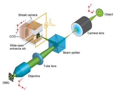
**Fig. 22.** Optical setup of compressed ultrafast photography (CUP). DMD, digital micro-mirror device. *Source:* Figure reprinted with permission from [209].
