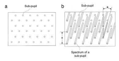
Fig. 4. Integral imaging spectrometry using hyperpixels. a. Image of undispersed sub-pupils after pinhole filtering. b. Image of spectrally dispersed subpupils. Source: Figure reprinted with permission from [32].
