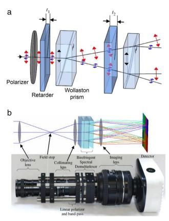
**Fig. 8.** Image-replicating imaging spectrometry (IRIS). a. Birefringent spectral demultiplexor. b. Optical setup. *t*<sub>1</sub>, *t*<sub>2</sub>, thickness of retarders. *Source:* Figure reprinted with permission from [35].
