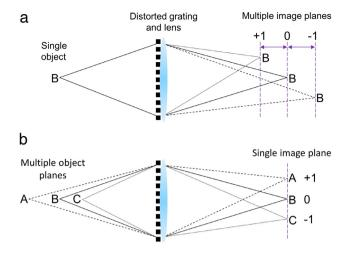
**Fig. 15.** Use of a distorted grating in an imaging system. a. When a single object is imaged by a distorted grating and lens, different diffraction-order images are formed at different image planes. b. When multiple objects at the correct depths are imaged by the same system, their different diffraction-order-associated images are formed on the same image plane but at different lateral locations. *Source:* Figure adapted with permission from [124].
