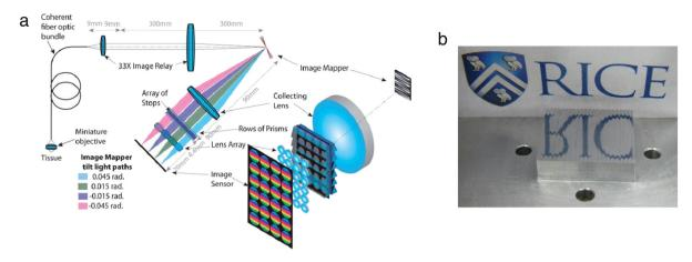
**Fig. 3.** Image mapping spectrometry (IMS). a. Optical setup. b. Photograph of an image mapper. *Source:* Figures reprinted with permission from [45] and [17].
