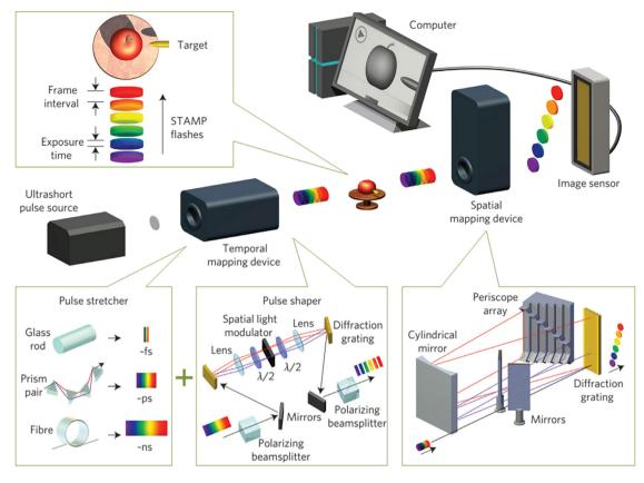
**Fig. 18.** Sequentially timed all-optical mapping photography (STAMP). *Source:* Figure reprinted with permission from [26].
