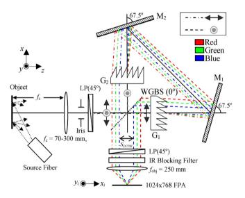
**Fig. 10.** Optical setup of a multispectral Sagnac interferometer. *G*<sub>1</sub>, *G*<sub>2</sub>, diffraction gratings; LP, linear polarizer; M<sub>1</sub>, M<sub>2</sub>, mirrors; WGBS, wire-grid beam splitter. The dash-dotted and dashed lines represent two orthogonal polarization directions. *Source:* Figure reprinted with permission from [38].
