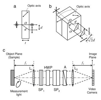
**Fig. 27.** Snapshot imaging polarimetry using Savart plates. a. Uniaxial birefringent crystal in a Savart plate. b. Savart plate. c. Optical setup. HWP, half-wave plate; L<sub>1</sub>, L<sub>2</sub>, lenses; SP<sub>1</sub>, SP<sub>2</sub>, Savart plates; A, analyzer. *Source:* Figure reprinted with permission from [229].
