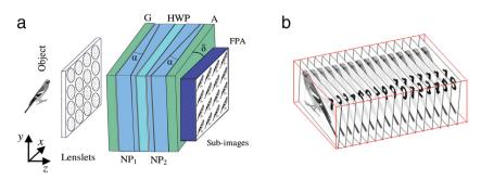
**Fig. 9.** Snapshot hyperspectral imaging Fourier transform spectrometry (SHIFT). a. Optical setup. b. 3D interferogram. A, analyzer; FPA, focal plane array; G, polarizer; HWP, half wave plate; NP<sub>1</sub>, NP<sub>2</sub>, Nomarski prims. *Source*: Figure adapted with permission from [64].
