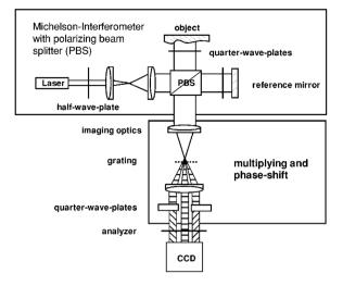
**Fig. 16.** Optical setup of a parallel phase-shifting digital holography technique. *Source:* Figure reprinted with permission from [172].
