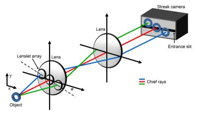
**Fig. 20.** Optical setup of parallel streak imaging using a lenslet array. *Source:* Figure adapted with permission from [200].
