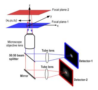
**Fig. 13.** Dual-camera optical setup for simultaneous two-plane imaging. *Source:* Figure reprinted with permission from [118].
