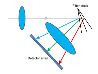
Fig. 6. Imaging spectrometry using a filter stack.
