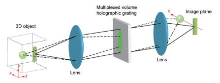
**Fig. 14.** Snapshot volumetric imaging using a multiplexed volume hologram. *Source:* Figure adapted with permission from [121].
