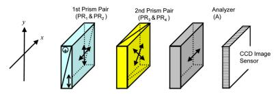
Fig. 26. Schematic of a device using four wedged birefringent prisms and an analyzer to perform complete imaging polarimetry. PR, prism pair. *Source:* Figure reprinted with permission from [66].
