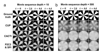
Fig. 24. Comparison of reconstruction reliability in CUP, CACTI, and P2C2 and SPI. The reconstructed movie sequence depths are 10 and 500 frames for a and b, respectively.
