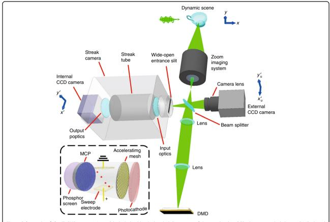
Fig. 2 Schematic of the T-CUP system. Inset (black dashed box): detailed illustration of the streak tube. CCD charge-coupled device, DMD digital micromirror device, MCP micro-channel plate
