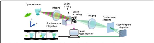
Fig. 1 Principle of operation for T-CUP. The beam paths for time-unsheared and time-sheared views are illustrated using magenta and green colors, respectively
