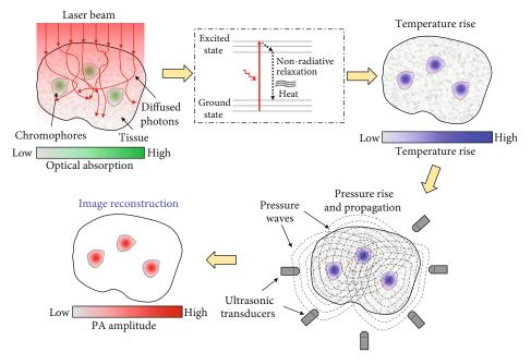
FIGURE 1: The principle of PAT.
