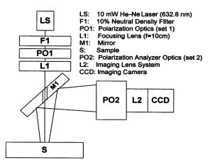
Fig. 1. Schematic diagram of experimental setup used for the Mueller matrix imaging of the diffusely backscattered light from the sample.
