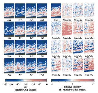
Fig. 2. (a) Raw OCT images with normalized intensity. All the images share the same color map. The size of each image is 750  $\mu$ m  $\times$  500  $\mu$ m. The bottom boundary in each image represents the incident surface of the bone sample. (b) Mueller matrix images. The Mueller matrix images (except  $M_{00}$ ) are normalized to  $M_{00}$  and share the same color map.
