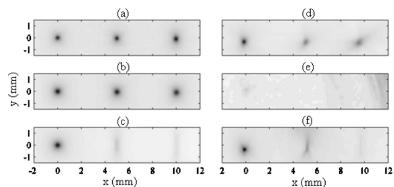
FIG. 3. Simulated images of point targets acquired using (a) a virtual detector, (b) a point detector, and (c) a finite-aperture detector. Experimental images of point targets acquired using (d) a virtual detector, (e) a point detector, and (f) a finite-aperture detector.
