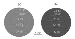
FIG. 4. Experimental images of line targets acquired using (a) a virtual detector and (b) a finite-aperture detector. Values of SNRs were evaluated in the middle of the lines.
