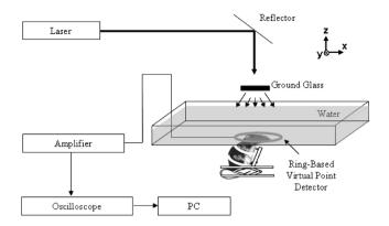
Fig. 1 Setup for photoacoustic tomography of the rat cerebral cortex.
