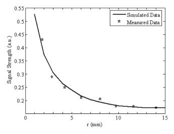
**Fig. 3** The signal strength of a point on a line target as a function of the distance *r* between the scan center and the center of the virtual point detector. The solid line represents the simulated data, and the asterisks represent the measured data.
