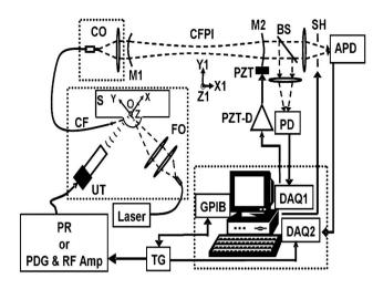
**Fig. 1** Schematic of the experimental setup: APD, avalanche photodiode; BS, beamsplitter; CF, collecting fiber; CFPI, confocal Fabry-Perot interferometer; CO, coupling optics; DAQ, data acquisition board; FO, focusing optics; M1, M2, mirrors inside the cavity; PD, photodetector; PDG, pulse delay generator; PR, pulser-receiver; PZT, piezoelectric transducer; PZT-D, piezoelectric transducer driver; RF Amp, RF amplifier; S, sample; SH, shutter; TG, trigger generator; UT, ultrasonic transducer.
