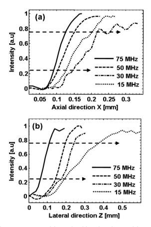
**Fig. 4** Measurement of the axial and lateral resolutions of the UOT images shown in Fig. 3, obtained with all four high-frequency ultrasound transducers. (a) Axial edge spread functions, and (b) lateral edge spread functions of UOT signals for respective high-frequency ultrasound transducers.
