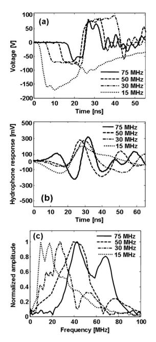
**Fig. 2** (a) Driving pulses of all four ultrasound transducers. (b) Hydrophone responses of the transducers in response to respective driving pulses. (c) Frequency spectra of (b).
