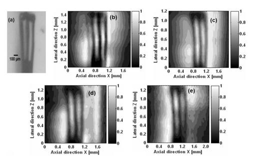
Fig. 6 Imaging of three optically absorbing objects located 2.0 mm inside the tissue-mimicking phantom along the ultrasound propagation direction, with all four high-frequency ultrasound transducers. (a) Photograph of three optically absorbing objects. B-scan UOT images of (a) obtained with (b) 15-MHz transducer, (c) 30-MHz transducer, (d) 50-MHz transducer, and (e) 75-MHz transducer.
