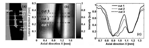
**Fig. 5** Imaging of high-resolution axial target located 2.0 mm inside the tissue-mimicking phantom using 75-MHz transducer. (a) Photograph of axial resolution target marked with two different sizes of gap; cut 1=75  $\mu$ m and cut 2=30  $\mu$ m. (b) B-scan UOT image of (a) marked with the respective cuts and cut 3=15  $\mu$ m. (c) Three 1-D axial profiles, from the intensity data in (b), corresponding to three different cuts shown in (b).
