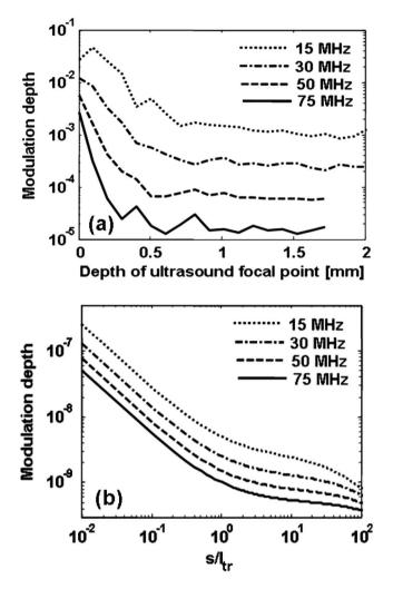
**Fig. 7** (a) Experimental measurement of modulation depth as a function of the ultrasound focal point location inside the chicken breast tissue for all four high-frequency ultrasound transducers. (b) Numerical simulation of modulation depth as a function of the average number of scattering events s/I, for ultrasound frequencies of 75 MHz, 50 MHz, 30 MHz, and 15 MHz.
