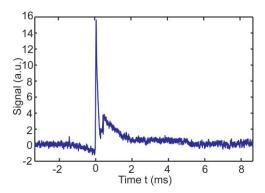
**Fig. 2** An example waveform of the detected TRUE signal from a 5-mm thick scattering sample with scattering coefficient  $\mu_s = 10 \text{ mm}^{-1}$  and scattering anisotropy g = 0.9. The peak from 0 to 0.2 ms is the TRUE signal, and the subsequent fluctuation comes from electronic coupling noise.
