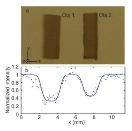
**Fig. 6** TRUE image of a sample with an optical thickness of 70 with the 2.0 MHz HIFU transducer. (a) Photograph of the sample embedded with two absorption objects (Objs 1 and 2) in the middle plane after dissection. The widths of the two objects were 2.0 and 1.7 mm, respectively, and their lengths and thicknesses were all 6.0 mm and z = 0.7 mm. The full dimensions of the sample were  $60 \times 60 \times 7$  mm<sup>3</sup>. (b) A TRUE image of the sample.
