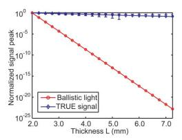
**Fig. 3** Comparison of the experimental TRUE optical signal (with error bar) and the computed ballistic light signal at varied thickness  $\it L$ . The TRUE signal had a much smaller decay rate, while ballistic light decays as a negative exponential function of thickness.
