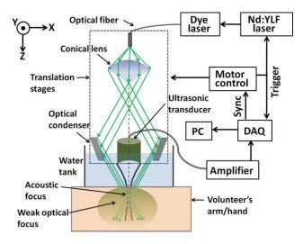
**Fig. 1** Schematic of the photoacoustic microscope used in the described experiments.
