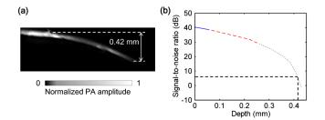
**Fig. 4** Measurement of the penetration depth of the submicron-resolution PAM. (a) A human hair inserted obliquely into chicken leg tissue is imaged clearly down to 0.42 mm beneath the tissue surface. (b) Signal-to-noise ratio (SNR) of the hair versus imaging depth. Dashed lines indicate 6 dB SNR at 0.42 mm imaging depth. The data from the three focal depths 0.04, 0.1, and 0.3 mm are denoted by solid, dashed, and dotted line types.
