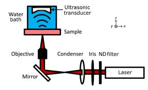
**Fig. 1** Schematic of the photoacoustic microscope (PAM). A laser pulse is attenuated by a neutral density (ND) filter, spatially filtered, and then focused by the objective onto the nerve sample. Optical absorption leads to the generation of photoacoustic waves, which are measured using an ultrasonic transducer. An image is generated by two-dimensional raster scanning of the sample.
