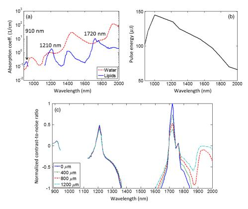
**Fig. 3** (a) The absorption coefficients of water and lipids versus wavelength. Three peaks of positive contrast for lipids occur at 910 nm, 1210 nm, and 1720 nm. (b) The pulse energy of the laser measured at each wavelength. (c) The normalized contrast-to-noise ratio as a function of wavelength estimated for several depths: 0, 400, 800, and 1200  $\mu$ m.
