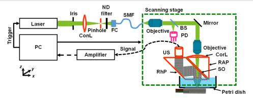
**Fig. 1** Schematic of OR-PAM. BS, beam splitter; ConL, condenser lens; CorL, correction lens; FC, fiber coupler; ND, neutral density; PD, photodiode; RAP, right-angle prism; RhP, rhomboid prism; SMF, single-mode fiber; SO, silicone oil; and US, ultrasonic transducer.
