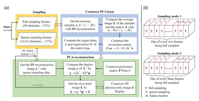
Fig. 1 Illustration of 3-D PCA-PACT. (a) Flowchart of the reconstruction process and (b) illustration of two kinds of sampling modes.
