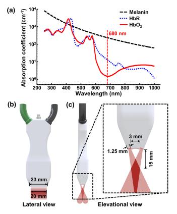
**Fig. 1** Absorption spectra of melanin and hemoglobin, and the front and side views of the handheld probe for LA-PAT. (a) Absorption spectra of melanin and hemoglobin. An excitation wavelength of 680 nm was chosen for the optimal CNR. (b) Lateral view of the handheld probe. (c) Elevational view of the handheld probe with a zoomed-in view.
