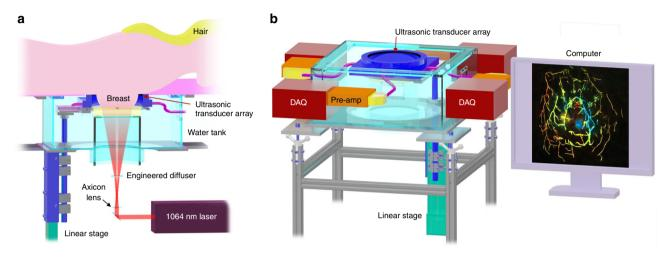
**Fig. 1** Representations of the SBH-PACT system. **a** Perspective cut-away view of the system with data acquisition components removed. **b** Perspective view of the system with patient bed and optical components removed. DAQ data acquisition system, Pre-amp pre-amplifier circuits
