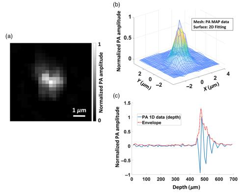
**Fig. 2** Lateral and axial resolutions of the MF-UV-PAM system. (a) A representative MAP image of the photoacoustic signal of a gold nanoparticle. (b) Isotropic 2-D Gaussian fitting of the MAP image in (a). (c) Reconstructed 1-D image along the depth direction of the gold nanoparticle in (a) and its Hilbert transformation.
