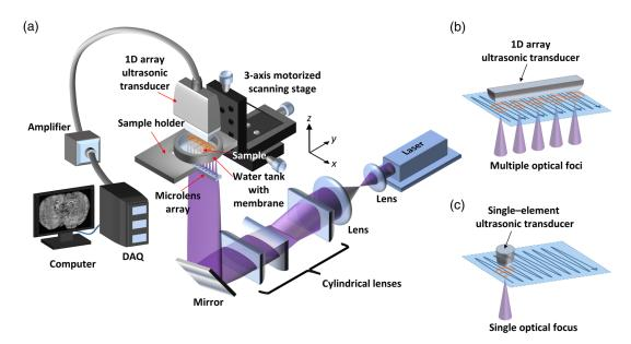
**Fig. 1** Schematic of multifocal ultraviolet laser photoacoustic microscopy (MF-UV-PAM) system and a comparison with conventional ultraviolet laser photoacoustic microscopy (UV-PAM). (a) Schematic of MF-UV-PAM. (b) The conventional UV-PAM system with a single optical focal point. (c) MF-UV-PAM system with multiple optical focal points.
