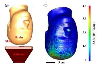
Fig. 2. (a) Simulation model of a head orienting toward the horn antenna. (b) SAR distribution with a peak SAR amplitude of  $4\times10^{-2}$  W/kg.
