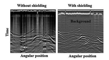
Fig. 4. Diagrams of TAT signals acquired before and after shielding.
