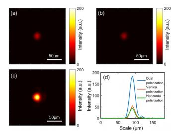
**FIG. 4.** Experimental results of focusing through a piece of thick chicken tissue. (a)–(c) are images of the foci captured by the CCD when only the vertical polarization component, only the horizontal polarization component, and both components are phase-conjugated, respectively. (d) The line profiles of the foci along the central rows of (a)–(c).
