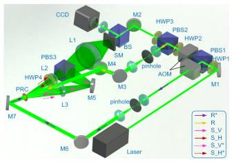
**FIG. 3.** Schematic of the experimental setup for dual-polarization AOPC. AOM, acousto-optic modulator; BS, beam splitter (nonpolarizing); CCD, charge-coupled device camera; HWP, half-wave plate; L, lens; M, mirror; PBS, polarizing beam splitter; PRC, photorefractive crystal; R, reference beam; S\_V, vertically polarized signal beam; S\_H, horizontally polarized signal beam; SM, scattering medium.
