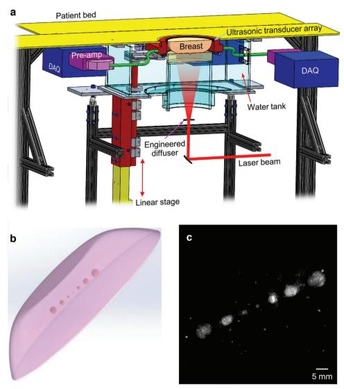
**Figure 1.** Schematic of the SBH-PACT and breast phantom imaging. a) Perspective cut-away view of the SBH-PACT breast imaging system. DAQ, data acquisition module; Pre-amp, preamplifiers. b) Sketch of the breast-mimicking phantom. c) Maximum-amplitude-projection (MAP) of the breast phantom image acquired by SBH-PACT, which revealed the smallest tumor phantom (1-mm diameter). The bright dots in the image background were caused by air bubbles embedded in the phantom.
