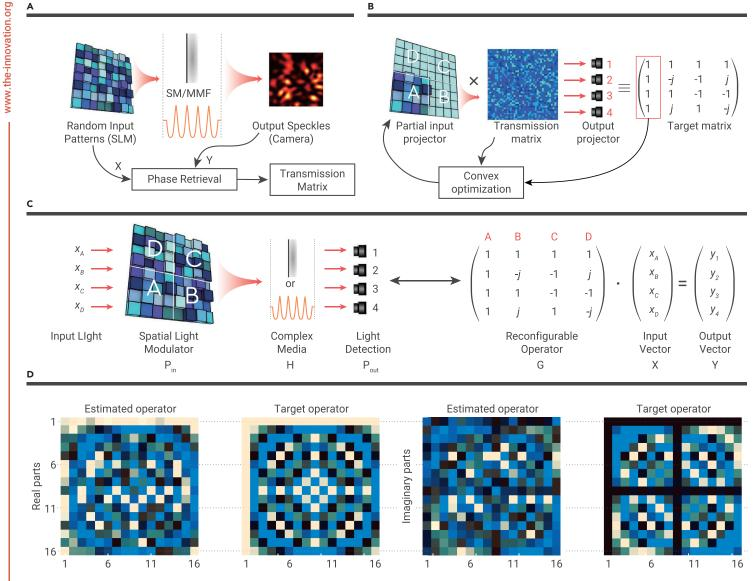
Figure 4. Reconfigurable optical linear operations (A) System calibration. (B) Optimal input projection calculation. (C) Analog computation. (D) Experimental results of a 16 x 16 discrete Fourier transform. All images are from Matthès et al.<sup>48</sup>
