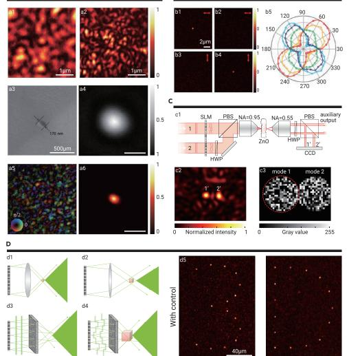
volume display with a precalculated pattern displayed on the SLM with significantly extended viewing angle and image size (Figure 3D). Yu et al. showed that the product of viewing angle and image size can be enhanced by a factor of 2.600 by adding two holographic diffusers compared with the case of using a single wavefront modulator only.<sup>138</sup> For example, as shown in Figure 3D, two characters "3D," with 15 foci for
