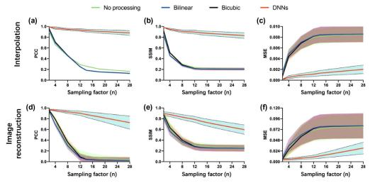
**Fig. 6.** Performance analysis of speckle interpolation and image reconstruction. (a)–(c) The PCC (a), SSIM (b), and MSE (c) between the interpolated speckles of interest and the original speckles ( $d_0$ -sampled). (d)–(f) The PCC (d), SSIM (e), and MSE (f) between the corresponding reconstructed images and the target human face. The solid lines and the shadowed regions represent the mean value and the standard deviation, respectively, from the 2000 testing samples.
